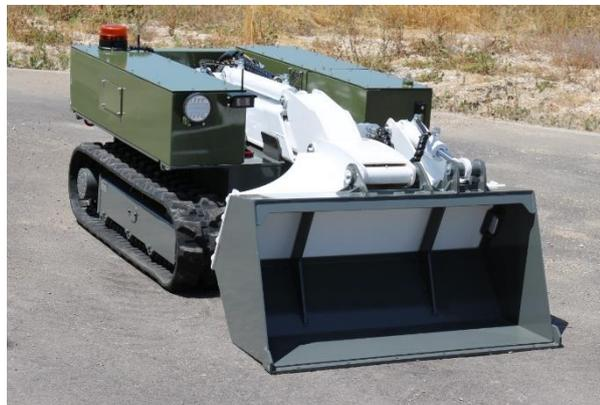
The *JOXE* machine is a hydraulically driven robot designed to perform work in confined spaces. The robot is designed to have a low height in order to access in confined spaces where conventional loader cannot access. Moreover the robot is equipped with a telescopic arm very useful to unload the material in boxes and to reach higher surfaces. The bucket is a clamshell bucket opened by an hydraulic cylinder.
